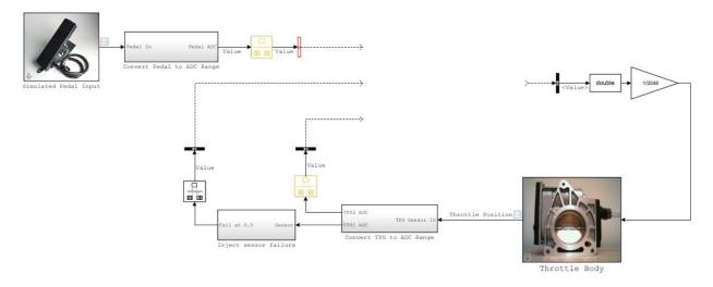
To connect the architecture model to the test harness, insert a Model block, and configure the Model block to reference the architecture model.
