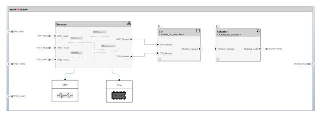
Here is a test harness model for simulating the architecture model autosar\_tpc\_composition. The test harness contains a plant model with a pedal input block and signals that correspond with the architecture model require and provide ports. This model was adapted from example model autosar tpc system.
