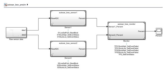
Sensor components autosar\_bsw\_sensor1 and autosar\_bsw\_sensor2 each contain an Initialize Function block, which calls the NvM service interface NvMService. The calls are implemented using the Basic Software library block NvMServiceCaller. Each block is configured to call the NvMService operation ReadBlock. The ReadBlock calls use client ports S1LowSetPoint and S2LowSetPoint. Here is the Initialize Function block for autosar bsw sensor1.
