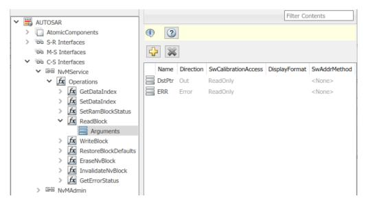
The software creates a client port with the default name NvMService. Unlike the C-S-interface, operation, and argument names, the client port name can be customized. The client port is mapped to the NvMService interface.
