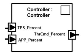
Use the MATLAB function createComponentAsModel to import the arxml description and create an initial Simulink representation of the AUTOSAR component.
