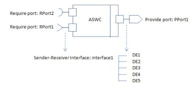
The AUTOSAR software component has a Require and Provide port that references the same Sender-Receiver Interface, Interface1. Although this interface contains data elements DE1, DE2, DE3, DE4, and DE5, the component does not utilize all of the data elements.
