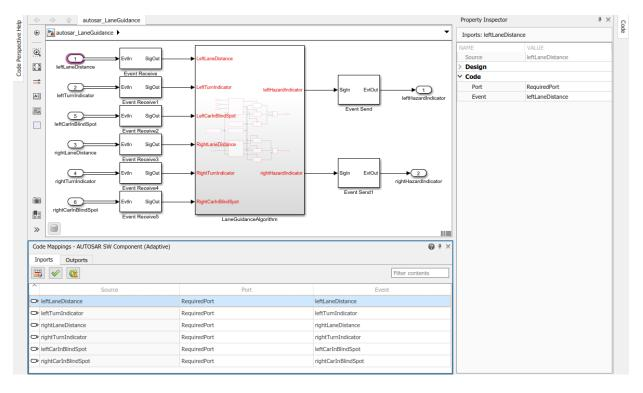
The Code Mappings editor provides in-canvas access to AUTOSAR mapping information, with batch editing, element filtering, easy navigation to model elements and AUTOSAR properties, and model element traceability.
