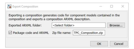
As the architecture model builds, you can view the build log in the Diagnostic Viewer. First the component models build, each as a standalone top-model build. Finally, composition arxml is exported. When the build is complete, the current folder contains build folders for the architecture model and each component model in the hierarchy, and the specified zip file.
