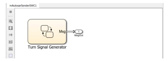
Here is the logic implemented in the Turn Signal Generator chart. The chart has four states – ActivateLeft, DeactivateLeft, ActivateRight, and DeactivateRight. Each state contains entry actions that assign a value to message data and send a message. (See "Communicate with Stateflow Charts by Sending Messages" (Stateflow).) Periodic timing drives the message output.
