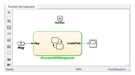
Here is the logic implemented in the ProcessHMIRequests chart. ProcessHMIRequests contains states HMIRequestProcessing, LeftTurnSignal, and RightTurnSignal. (This receiver chart is similar to chart HMILogic in the 1-to-1 and N-to-1 simulation examples.)
