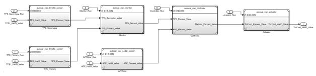
Signal lines between component models represent AUTOSAR assembly connectors. Signal lines between component models and data inports and outports represent AUTOSAR delegation connectors.
