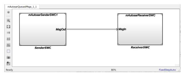
Models mAutosarSenderSWC1 and mAutosarReceiverSWC are the same sender and receiver components configured in "Configure AUTOSAR Sender and Receiver Components for Queued Communication" on page 4-147 and implemented in "Implement AUTOSAR Queued Send and Receive Messaging" on page 4-150. Composition-level model mAutosarQueuedMsgs\_1\_1 includes them as referenced models and connects sender component port MsgOut to receiver component port MsgIn.
