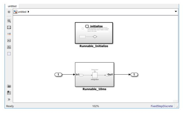
In this example, the created model is a starting point for developing a software component for the AUTOSAR Classic Platform.
