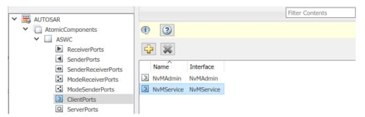
The Code Mappings editor maps the NvMService function caller block to AUTOSAR client port NvMService and AUTOSAR operation ReadBlock.
