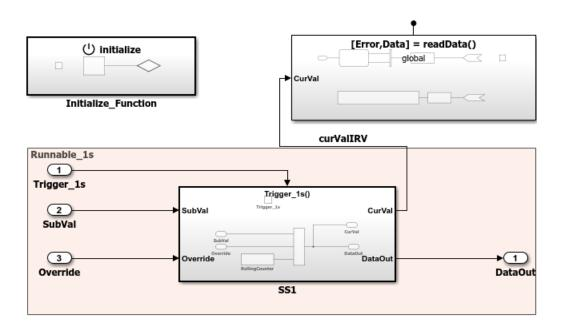
If your AUTOSAR software component design contains periodic runnables, you must decide whether your component requires a rate-based or function-call based modeling approach. Before you create an initial Simulink representation of your AUTOSAR component, designate how to model periodic runnables:
