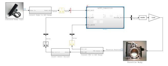
The test harness model is now ready to be simulated. Click **Run**. When you simulate the application, the throttle position scope indicates how well the throttle-position control algorithms in the architecture model are tracking the accelerator pedal input.
