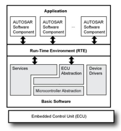
The Classic Platform uses a virtual functional bus (VFB) to support hardware-independent development and usage of AUTOSAR application software. The bus consists of abstract representations of RTEs for specific ECUs, decoupling AUTOSAR software components in the Application layer of the architecture from the architecture infrastructure. AUTOSAR software components and the bus communicate by using dedicated ports. You configure
