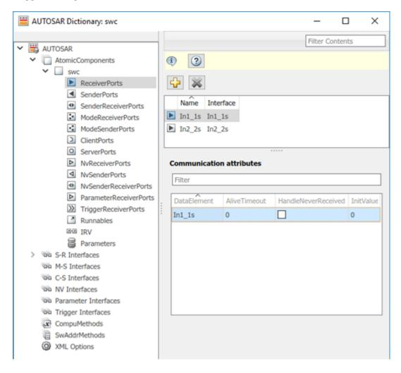
The AUTOSAR Dictionary displays the mapped AUTOSAR component and its elements, communication interfaces, computation methods, software address methods, and XML options. Use the dictionary to configure AUTOSAR elements and properties from an AUTOSAR component perspective.
