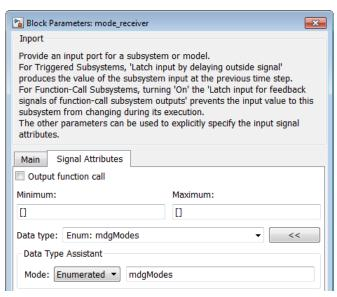
3 To specify the mapping of the Simulink inport to the AUTOSAR mode-receiver port, use the Code Mappings editor (or equivalent AUTOSAR map functions).
