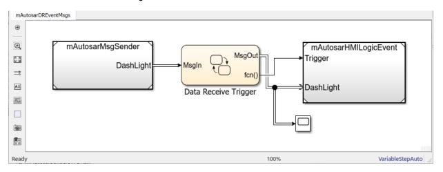
Composition-level model mAutosarDREEventMsgs includes a sender component and a receiver component as referenced models. It connects the sender message port DashLight to intermediate Data Receive Trigger logic, which in turn connects to receiver message port MsgIn and function trigger port Trigger.
