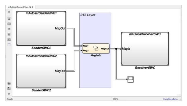
Composition-level model mAutosarQueuedMsgs\_N\_1 includes two sender components and a receiver component as referenced models. It connects the sender component MsgOut ports to intermediate MsgJoin processing logic, which in turn connects to a receiver component MsgIn port.
