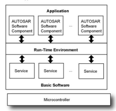
Automobile manufacturers, suppliers, and tool developers jointly develop components of the Application layer. The standard refers to the components as AUTOSAR software components. They interact with the Run-Time Environment layer. The Run-Time Environment layer enables communication between:
