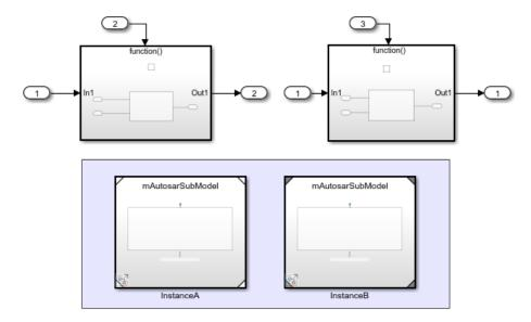
Open the submodel standalone, that is, in a separate model window. In the model window, from the **Apps** tab, open the AUTOSAR Component Designer app. If the submodel is mapped, it opens in the AUTOSAR code perspective.
