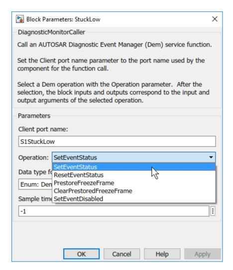
Monitor component autosar\_bsw\_monitor contains a call to the Dem service interface DiagnosticMonitor and four calls to the DEM service interface DiagnosticInfo.
