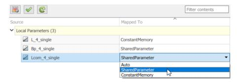
In this example, COM\_AXIS breakpoint object Bp\_4\_single and lookup table object Lcom\_4\_single are mapped to AUTOSAR SharedParameters. All instances of the AUTOSAR software component share the COM\_AXIS parameters.
