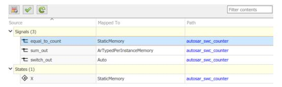
The **Signals/States** tab, **States** node, lists each configurable Simulink block state that you can map to an AUTOSAR variable. You can map a Simulink block state by selecting
