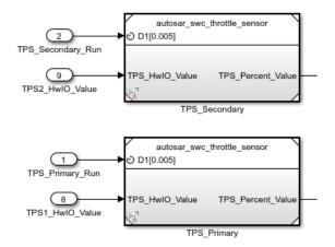
If you open autosar\_composition, you can right-click the Model blocks that represent instances of autosar\_swc\_throttle\_sensor. If you open up each Model block dialog box, **Instance Parameters** tab, and view them together, notice that each Model block uses a different value for the per-instance parameter.
