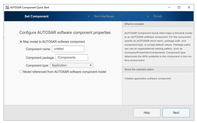
4 Work through the quick-start procedure. If necessary, refer to "Create Mapped AUTOSAR Component with Quick Start" on page 3-2. When you click **Finish**, your model opens in the AUTOSAR code perspective. To continue configuring the component model, see "AUTOSAR Component Configuration" on page 4-3
