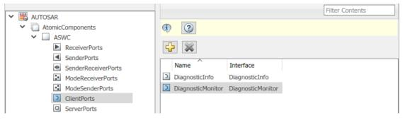
The Code Mappings editor maps the DiagnosticMonitor function caller block to AUTOSAR client port DiagnosticMonitor and AUTOSAR operation SetEventStatus.
