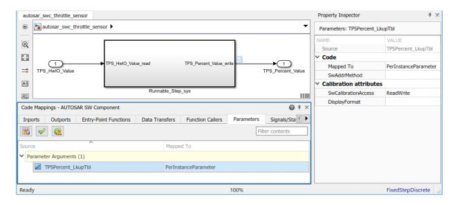
AUTOSAR example model autosar\_composition is a composition model that contains several components, including two instances of component model autosar swc throttle sensor.
