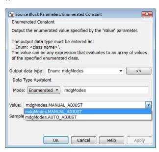
Apply the enumeration data type to a Simulink inport that represents an AUTOSAR mode-receiver port. In this Inport block dialog box, enumerated type mdgModes is specified as the inport data type.
